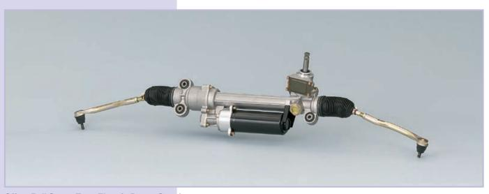
Offset Ball Screw Type Electric Power Steering
