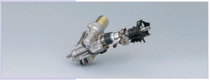
**Column Type Electric Power Steering**Column type EPS with mid-tilt mechanism for small cars.
